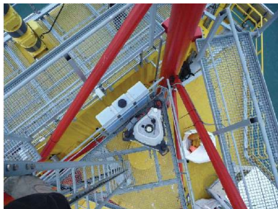
Figure 7 - LiDAR located within the lattice structure of the Meteomast IJmuiden offshore met mast [source: ECN]
